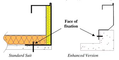
Allother places for attachment may Cause water leakage.
